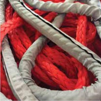
POLYESTER WOVEN SLEEVE IS STRONG, RESISTANT TO UV LIGHT AND CHEMICALS, KIND ON THE HANDS AND STRETCHES JUST MODERATELY WHEN LOADED AND IDEAL FOR PROTECTING SPLICED EYES .THIS IS THE FIBER TO CHOOSE IN ANY APPLICATION WHERE ULTIMATE PERFORMANCE OR MINIMUM WEIGHT IS NOT ABSOLUTELY ESSENTIAL. IT IS AVAILABLE IN DIFFERENT COLORS.
